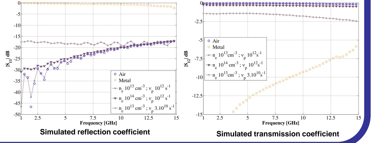
densities ( $n_e = 10^{14} \text{ cm}^{-3}$  and  $n_e = 10^{13} \text{ cm}^{-3}$ ).  $\circ$ Very low pressure discharge (n<sub>e</sub> = 10<sup>13</sup> cm<sup>-3</sup>; v<sub>p</sub> = 10<sup>10</sup> s<sup>-1</sup>). •Higher  $\omega_p$  /  $v_p$  ratio: more influence over RF parameters.
